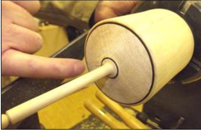
Mark the ring diameter plus a 1/4" onto the block left in the lathe, and commence reducing all that section into a spindle of the correct diameter to fit snugly (without binding, through the drilled holes in the ring.
