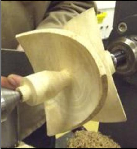
Try working the other bowl from the headstock side if you have enough room, but if not, turn the piece round on the lathe and work on the tail stock side. The net result will be that you have 2 three cornered bowls, joined back to back, each with a central spigot.
