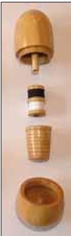
I proceeded with the usual method for box making by roughing down between centres, then with the blank in the chuck, I parted through for the lid and base. I hollowed the lid first, and chased the female thread, before forming part of the outside shape.
