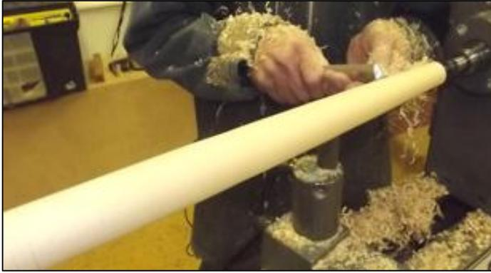
The 4 Maple legs started life as 22" long blanks of 50mm square timber. With a leg mounted between a steb and a live centre, it was rounded off with a spindle roughing gouge to about 48mm diameter. Reduce the first 10 " to 47mm, cut a 1" diameter spigot at the other end (to fit into the seat) and then taper the remaining timber from the 10" point to the spigot. You
