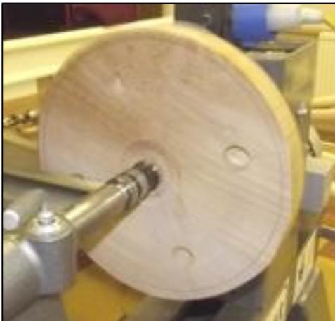
The stool we were to see consists of a turned Elm seat with four legs and stretchers made of Maple. Starting with the seat, mark the centre, the 12" diameter, and the location points for the 4 legs. Roger then showed us a platform he had made with a 12degree slope. This allows the leg holes to be drilled on a pillar drill, each being 1" diameter. With the seat then mounted between a live steb centre and the
