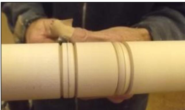
centre of each bead section, and roll over the edges, taking care to not lose the pencil line in the centre of each one. Also, you can roll over the edge of the foot at this stage. Mount the 4 legs in the seat, and rotate them to get the best grain presentation, then mark the face of each leg for the relevant long and short stretcher drilling. As you take the legs out of the seat, number them so that they go back in
