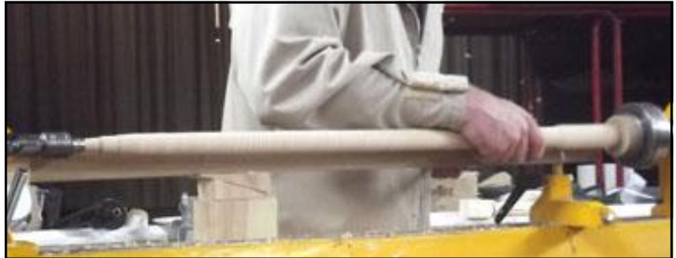
use of a home made tool rest which is the full length of the cane and the lathe, supported by the banjo at one end and is G-cramped to the tailstock at the other.
