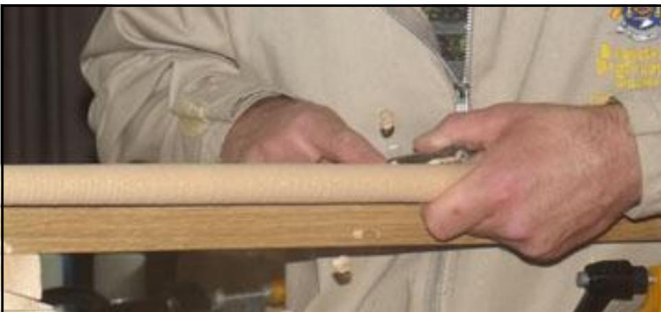
The wood used is Steamed Beech as it is easy to work, is stable and straight grained and because it is a relatively inexpensive hard wood. As he sprays the canes black for his client the rather plain grain pattern of Beech is not
