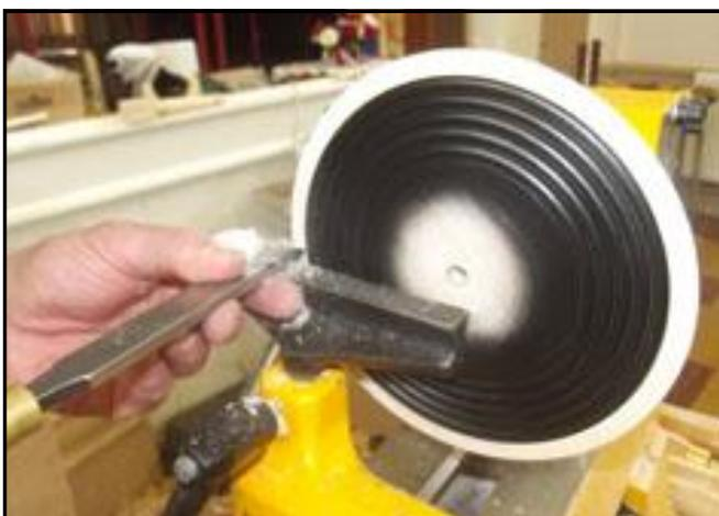
Now with the piece re-mounted using the spigot in the chuck, the top face was trued up with a few draw cuts, and a small amount of drop was added to the edge, producing quite a thin edge to the rim. Mark the face for edge and centre margins and the bowl section to be cut out later. Decorate between the pair of margin sections with a Sorby texturing tool if you have one. A cheaper option is a set of beads cut with an Ashley Iles beading tool.
