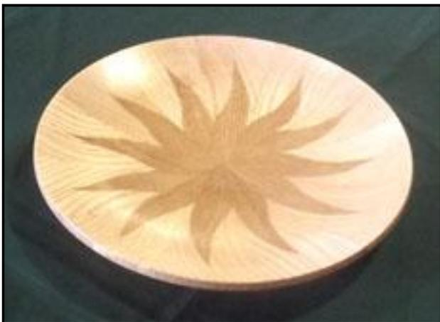
Once again, a stunning piece from Andy Moore, a staved platter made of Ash and Oak. Made by gluing the pieces together, then re-cutting the joints on a scroll saw, then re-assembly. A super finish with Simoniz car wax.
