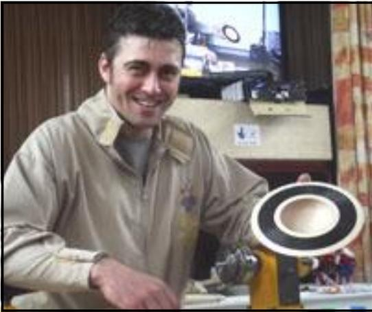
with. For the best effect, finish with an undercut at the rim flowing into a smooth cut right into the bottom of the bowl section.
