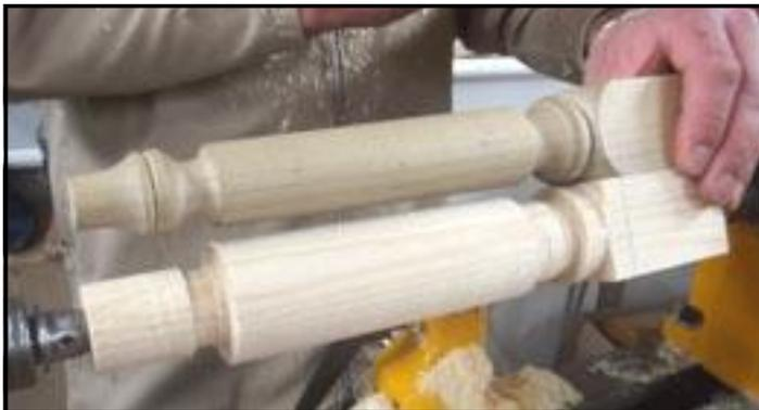
long point of a skew. This is to protect the corners on the square section at the top of the leg. The remainder of the leg was quickly rounded off with a spindle roughing gouge, and he then marked all the principal cuts from the template. Parting cuts were made to block out the main features, all of which were then cut and refined with a combination of spindle gouges and the skew.
