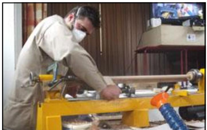
the bottom of the cane. Then with a spindle roughing gouge he did the majority of the shaping. Being left handed he starts at the right end of the cane and works to the left, offering support to the cane with his right hand. At this stage he is mostly focusing on taking away the corners and not worrying about cutting to the final depth.
