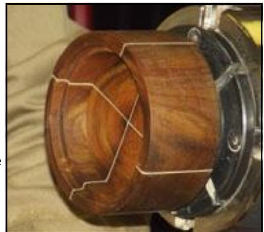
After cutting the lid recess, start cutting down the
