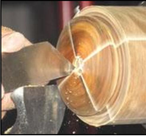
centres it was rounded off with a spindle roughing gouge and a dovetail spigot was cut. With this stage completed, the ball was mounted in the chuck.
