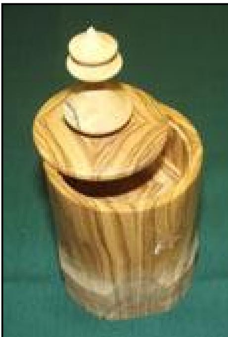
1) Make the finial in the chuck with tail stock support, don't forget to add a spigot at the base, sand, seal, polish, part off.
