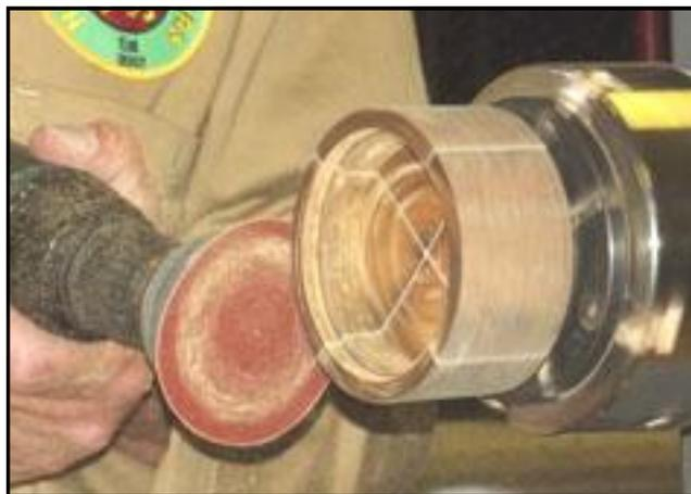
in the finial. Clean the recess in the Lignum with Acetone before gluing so as to reduce the oil content of the area.
