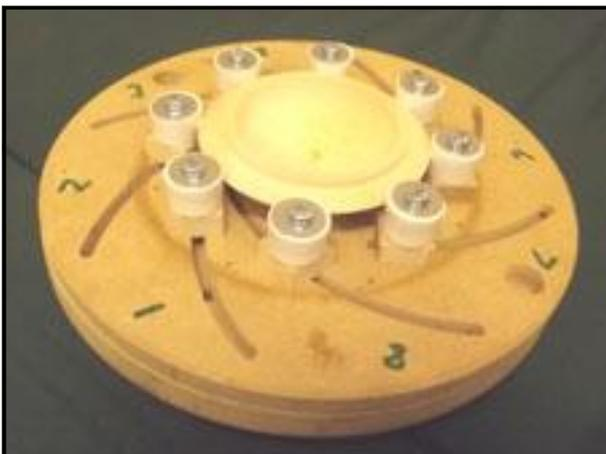
Three pieces from Ron Lansdell. First a Longworth chuck made from MDF and other bits and pieces. Well made, a clever piece of work.
