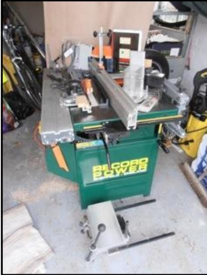
**Surface Planer:** Adjustable infeed table, maximum cut 4mm with extractor nozzle and bridge guard. Rotational speed 6300 rpm. Cutter block diameter 60mm. Length of infeed table 520mm. Maximum depth of cut per pass 4mm, width of cut 250mm. Blade brakes to stop in 4 seconds.
