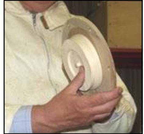
This was followed by a quick "re-demonstration" using a larger piece of Sycamore, during which Tom explained how he used a home made faceplate made of Sycamore and ply. This can be screwed into one of the rear recesses in the frame to help mount it in a chuck.
