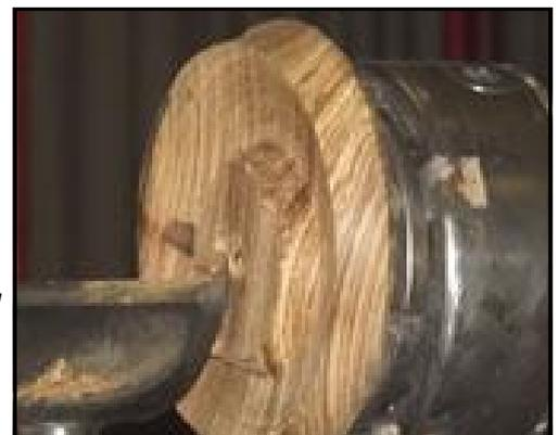
In summary, the back, the edge and the front face edge are all done on centre, the rear and front recess and cut through are all done off centre.
