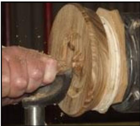
Last project for the evening was an offset mirror (or frame). Drill 2 holes for the screw chuck, about 1/2" apart. Make sure that the holes are either square to, or at right angles to the grain. Mount the piece for the back cuts "on centre" and do all as before. When trimming the edge, try to deal with the outer rim of the front face also, while things are on centre.
