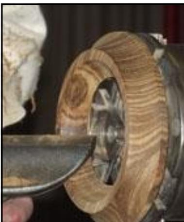
Tom explained that tool sharpness has a direct bearing on the final finish that you achieve. In reality, the sharper your tools are, the less sanding you need to do, hence, detail is easier to retain.
