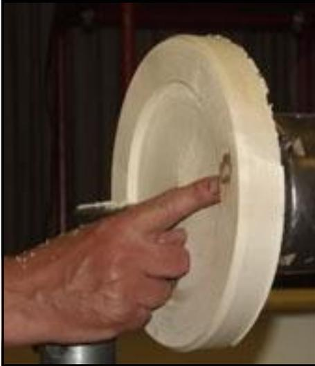
Take an accurate measurement of the "view through" aperture with a pair of callipers, then re-mount the piece the other way round on a regular chuck in expansion mode. Cut a simple curve into the edge, and skim the face. Use your calliper measurement to mark the diameter to be removed from the centre. Take care to NOT allow both legs of the calliper to be in contact with the wood. Remove the centre section as marked, keeping good track of where the chuck jaws are, meeting up with
