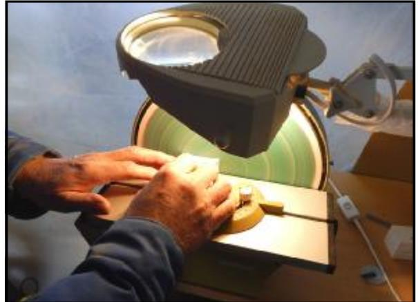
Glue 2 sets of 4 segments together using masking tape to hold the parts together. In half an hour or so you ought to be able to sand the remaining edges and glue the 2 half rings together.
