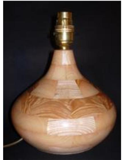
the bottom face of the next ring on your sanding disc with the table removed (wear a mask). Draw a new target circle on the assembly, glue on the next ring, and let the weight of the chuck hold everything in place as before. Repeat this process all the way up the vessel until you get to the top ring.
