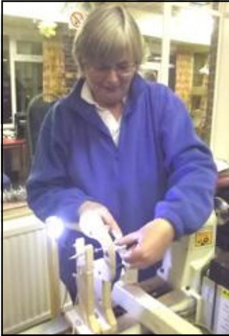
less than 2mm, and supports the work with temporary clamps mounted between the lathe bed rails. Natural string is used to support the work, having it strung around 3 pins to apply equal tension in all directions. Do not use man-made products for this, first they melt, and second, the piece you are turning will break.
