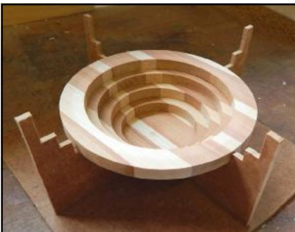
Also, I saw these rings. Cut from a laminated board. The first set have been cut on diameters of 4, 6, 8. and 10 cm (for instance), and the second set have been cut on diameters of 5, 7, 9, 11 cm. You then stack the rings in sequential sizes, i.e., 4, 5, 6, 7, etc. Clearly, this world is as broad as your imagination.
