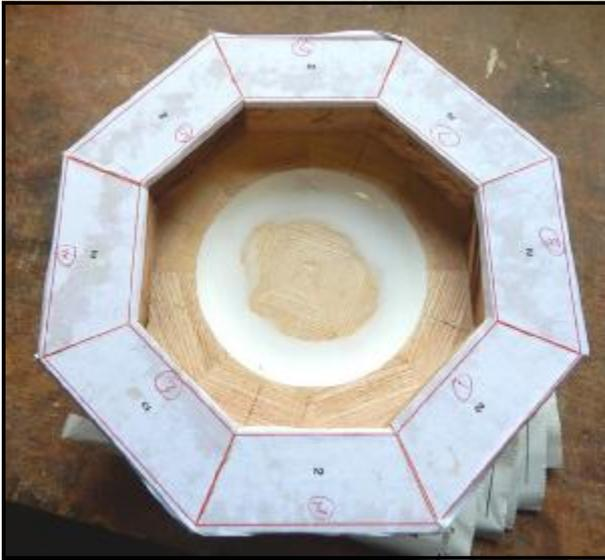
When everything is dry use white spirit to release the cutting patterns from the timber and a scraper and white spirit to clean the surface. Sand the open face of the assembly using a sheet of abrasive attached to a backing board. Sand
