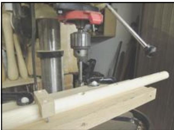
The legs are next and the same procedure is used, except that they are turned down to 1 1/4", the final diameter. Now we have to make a couple of jigs to assist drilling the holes and the mortises for the slats. They are simple and for the drilling you could just use a V block, however I made a jig approx. 24" long. It has a 5/8" groove in the middle of it and two side rails. The idea being that you place a leg on the groove, clamp it down, and drill the 5/8" holes
