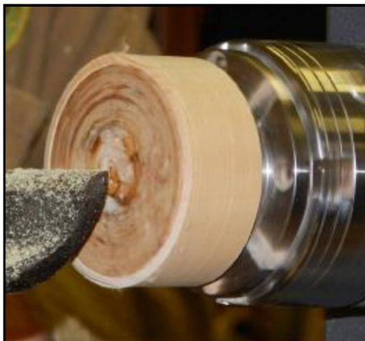
At the rim, the side wall was cut using a square end scraper leaving a thin step for the lid to sit on. Work continued in the bottom of the box and down the side wall until such time as the interior was complete, leaving a square corner in the bottom. This is John's preference, it allows a piece of felt to be inserted. Sand, seal and polish.
