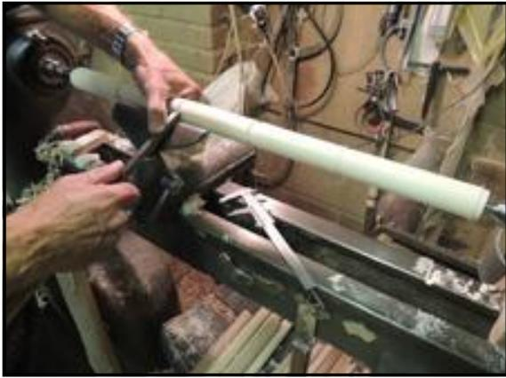
back are 3/8" thick. The front legs are at an angle of 9 degrees to the back legs. The whole chair was turned from Green Ash which had not been cut down very long, so was quite wet.
