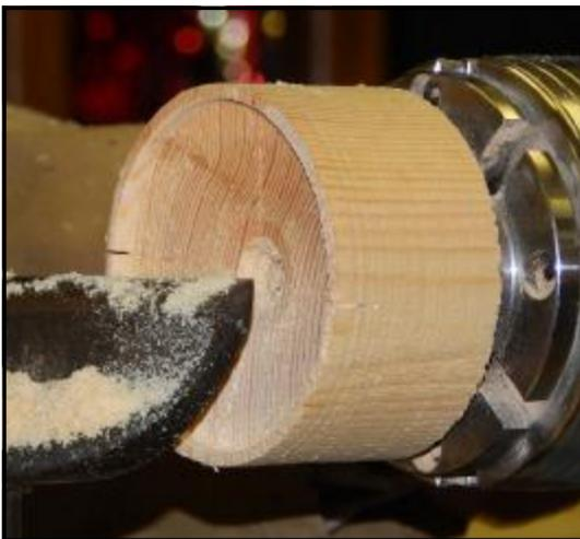
A lump of Sycamore was then mounted in the chuck. Having decided upon the box height, the waste was parted off, leaving the box blank in the chuck. It was rounded off leaving it about 10mm larger than the lid diameter. The outside face was trued up, and hollowing began with a round nose scraper, working from centre to rim. With an end grain box you should aim to leave at least 10mm in the bottom.
