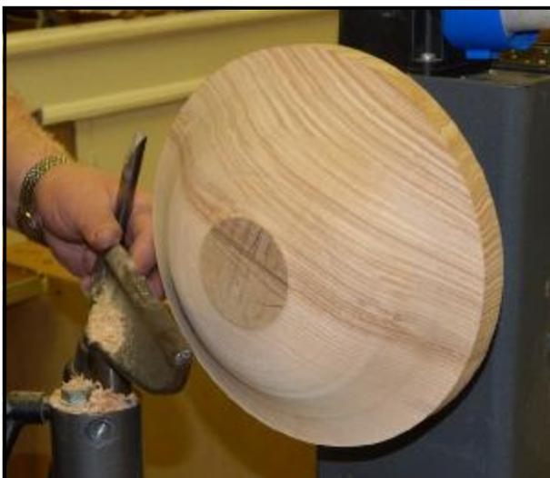
faceplate, a much safer method with a large, out of balance piece. Never attempt this type of work with either a spindle, or a spindle roughing gouge, you should only use a proper, well sharpened bowl gouge.
