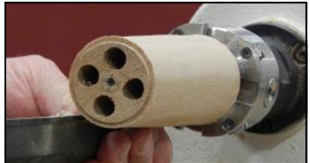
Bert started with a block of timber which had previously been drilled 1/2" diameter 4 times. The holes need to have varying depths of 4", 3.5", 3", and 2.5". Take care to get the holes equidistant from the centre of the blank, and sand the insides clean.
