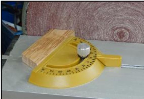
Having sanded the first end of each segment correctly with respect to the **LONG** edge of the timber, all that remains is to sand the second end to 40 degrees with respect to the first. This is all very easy when you have a tool which will measure angles for you with good repeatable accuracy.
