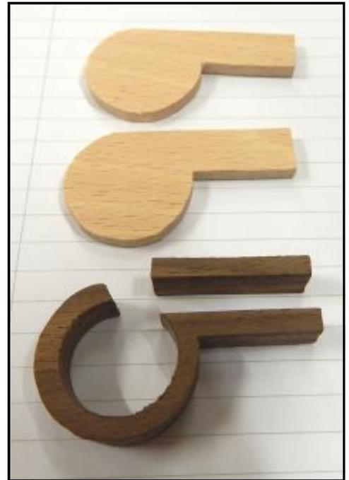
rectangular piece representing the upper part of the mouthpiece and the fourth was the only technical bit, as internally, it had been sawn to 1" diameter, and externally had been sawn and sanded to 1.25" diameter. Should you feel the need, you can also include a dried pea. No other description is needed,
