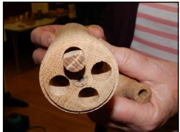
Turn the outside of the blank down so that the drilled holes have an external wall thickness of about 3/16". Face off the free end and cut a small recess on the end so that a cap can be fitted. Measure about 3/4" from the free end and turn away a tapered section (same shape as the tapered wedge on the police whistle). Turn about 2/3rds the way into the whistle chambers.
