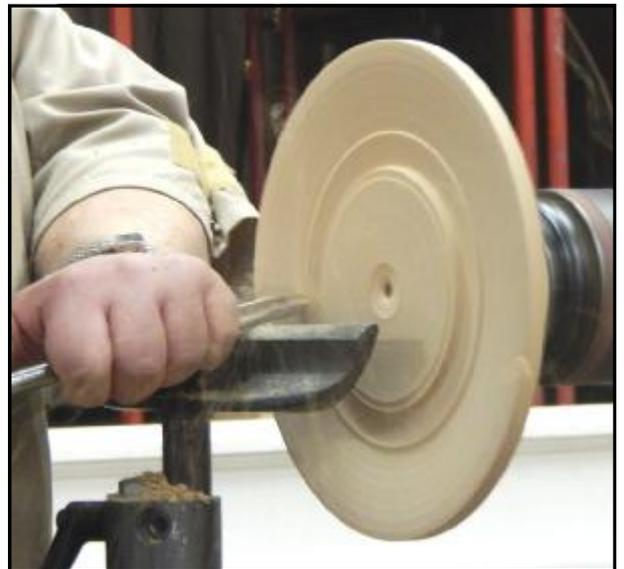
point of a skew, and test fit the chuck, it is better to find out now if the chuck does not fit well, and then adjust as necessary. With a square grind bowl gouge, use push cuts to finish the shape. A round skew with a curved cutting edge was used to give a perfect finish. Make sure you give the tool plenty of support with your fore arm and also, ensure that the burr is on the top edge of your tool because it is that burr that does the cutting.
