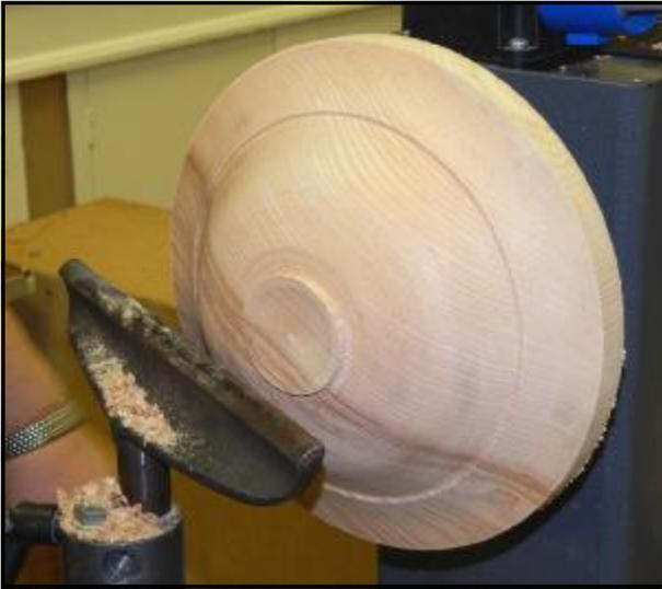
when the bottom shape approaches the top edge of the blank take a couple of straight cuts across the remaining edge to finally bring it all into balance.
