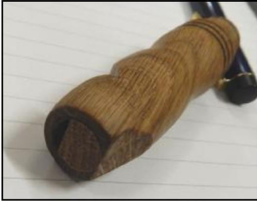
small block of wood, about an inch square and 4 to 5 inches long and drill one end 3/8" diameter 2 to 3 inches deep.
