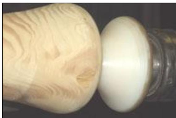
a large diameter live centre. Tom did this using an Axminster multi-tip live centre (p/n 718221/718222). The kit contains a small diameter face plate onto which you can mount many variations of a wooden support. With the form supported at both ends work on the outside of the
