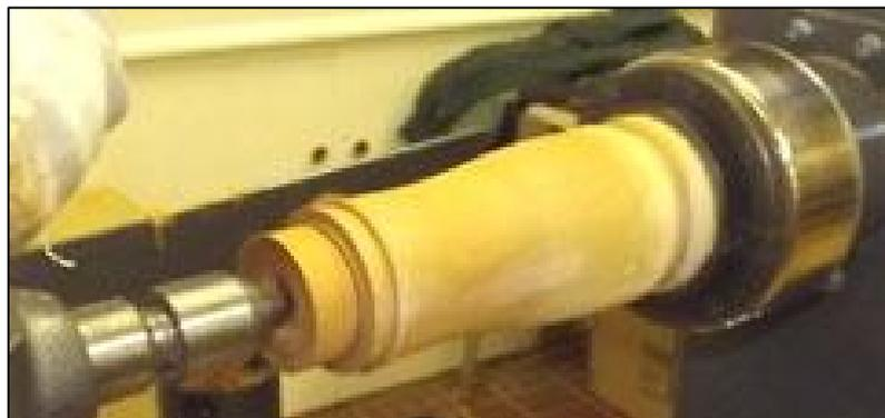
middle of the bottom end. Part in, and remove the end section of the piece. Keep this bit safe, it will eventually become a plug to close off the bottom end of your hollow form. When you do part this bit off, make sure you leave a witness mark on the main body of the piece. Ensure that the new tail end of the piece has a
