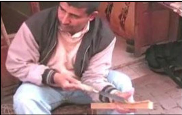
The equipment used clearly has its roots well and truly fixed in ancient times. The lathe bed consists of a couple of steel bars located in what would be loosely called the head and tail stock, the latter being made of wood. Laying across the top of the stocks is a third bar, this is the tool rest. Both the head and tail stock have a spike sticking out of them, they both act as live centres to mount a spindle blank between.
