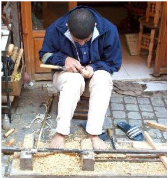
So, power is applied (the right arm) and with skew in left hand the right foot comes into play, controlling the chisel blade like you have never seen before, and within seconds, a whole section of the spindle has been rounded off. Parting 'V' cuts are made and in less time than it takes to write, a section has been reduced, opposing beads have been rolled, and all of a sudden, the section between them has been transformed into a captive ring.
