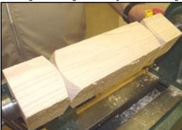
The evening's finale, a bit of spindle turning to demonstrate 'V' cutting with the skew (long point down) to create a pummel. The first cut was on the waste side, and don't forget that
