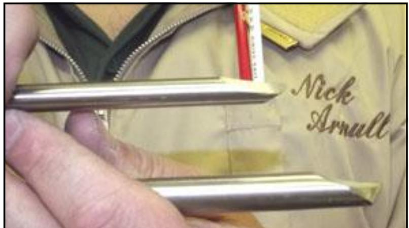
With scrapers, simply match the table angle to the tool angle and sharpen with long smooth movements across and round the tip of the blade.
