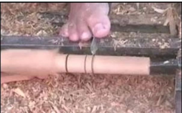
So, that takes care of work holding and motive power. Now we come to the cleaver bit, tool control and cutting. This is all done with a skew chisel held in the left hand, and controlled on the tool rest with the right foot. I picked up on an interesting comment on the internet about Mostopher, "is he left handed or right footed".
