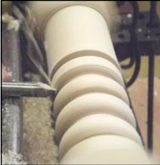
the cut will follow the line of the bevel. This was followed by waste removal with the spindle roughing gouge, you can use the side wings for a cleaner cut. The skew was then used with an ultra smooth planing cut and the point tool was used to help define the ends of the cut section. At this point we were treated to an (almost) heated discussion between Ivan and Nick as to whether or not the planed section was straight. Alan Calver sorted them both out by pronouncing it to be "proper straight".
