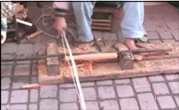
All adjustment is done via the tail stock (on the left). This is free to move left and right on the bed bars, and is kept in contact with the work piece with the left foot. Drive for the lathe is with a bow, manipulated back and forth with the right hand and arm.
