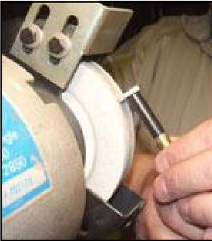
where the tool temper will be affected. The answer is simple, less pressure on the grinding wheel, and do it a bit quicker. Both of these will prevent heat build-up in the tool.
