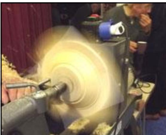
that the piece was badly out of balance, this was largely remedied with several heavy pull cuts, working from centre to rim. This was followed by cutting the corners back to about 45 degrees, which helps to protect them during the cutting of the main body of the platter.
