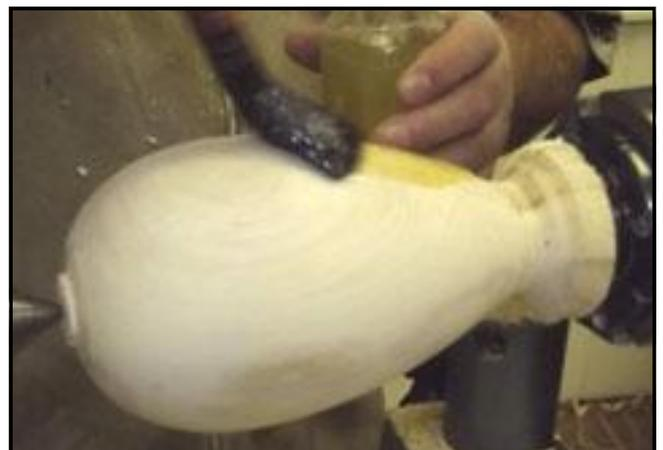
end". Re-mount in the chuck and refine the core shape until you are happy with it. With a re-sharpened gouge, make finishing cuts over the whole of the surface, followed by sheer scraping until you are happy with the entire line of the piece.
