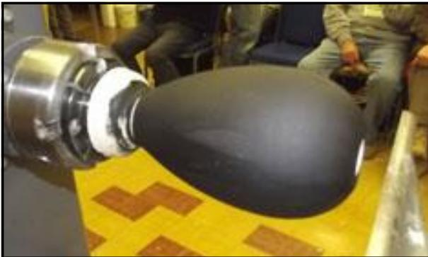
reduce the dust problem while you sand through the grits. Clean off the top surface, drill out the core of the vessel, and recess the neck to allow a turned neck piece to be inserted. Then, if you choose to, hollow out until your heart is content. Paint with black acrylic, and when dry, coat with spray lacquer.
