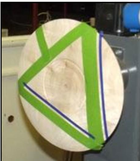
The spigot was then refined into a dovetail spigot. When you do this bit, make sure you cut it to an accurate size to match your chuck. If this is not accurate, it will affect the way the piece holds, and will be very easy to re-mount the piece off line.
