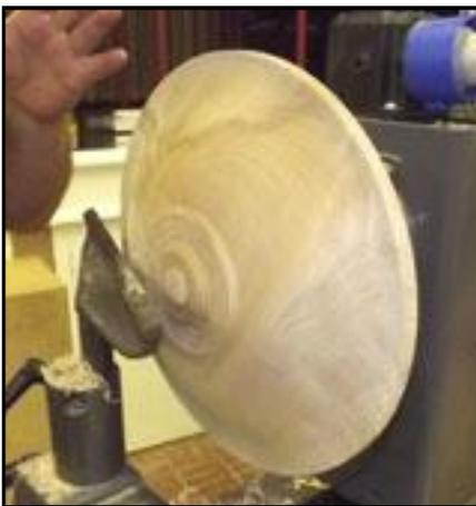
The evening started with a 14" blank of Sycamore on a screw chuck with some tailstock support. Using a heavy bowl gouge, Mick took a few cuts, first to true up the edge, and then in sheer mode, he cleaned up the first inch of the face nearest to the headstock, followed by the open face. In a matter of seconds the piece was in balance and running true. Coarse sheer cutting followed to produce a smooth ogee shape on the bottom, leaving a re-chucking spigot in the centre.
