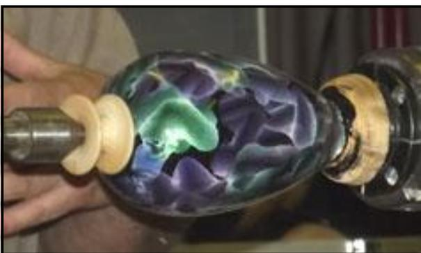
Turn a neck section to fit the recess you cut earlier. If necessary, cut several necks, and then choose which you like the best, sand and seal. With the neck glued in, the whole of the vessel can be coated in gloss lacquer, and deal with the base as you feel fit.
