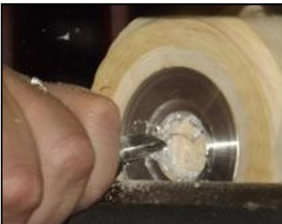
Like Mick Hanbury last month, the interior sanding was completed with a beeswax / oil mixture to give a near perfect result. This method is particularly useful when used in the bottom of boxes. With the box parted off, the lid section was mounted in the chuck and was used to make a jam chuck to reverse mount the box so as to allow the bottom to be finished off with a slight undercut. Add rings etc. to the underside.
