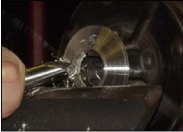
With the jam chuck still in the lathe, the edge was converted from a jam fit to a smooth fit, and a small recess was cut in the centre to fit a set of pin jaws on a second chuck. At this stage, the bulk of the waste on the lid was removed while a good hold on the blank could be maintained. This was followed by parting off a small section which now resembled a wide brimmed hat. Now re-mounted in the pin jaws, the top of the hat was rounded off.
