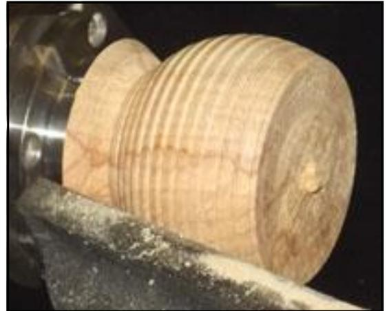
Simon very quickly noted that when turning he likes the lathe to run as fast as it can (within the bounds of safety). This will always give you a better finish. With a block of Spalted
