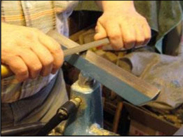
across the end of the blank in which to engage the drive centre. Look at your drive centre, is it damaged, if so, re-sharpen the prongs so they are able to penetrate the wood.
