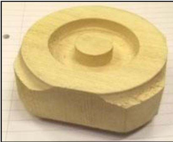
Rough down the exterior of the box to give the basic shape using a long grind bowl gouge, and complete the job with a square ground bowl gouge. This all seemed to happen in less time than it has taken me to type it. Using an Ashly Iles beading tool the whole of the exterior was beaded. A first pass, end to end to give the layout and basic cut, then a second pass to finish cutting all the beads to a perfect shape.
