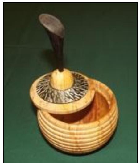
With a piece of African Blackwood in the pin jaws, it was turned down in a long sweeping curve measuring full diameter near the chuck, and 4mm at the free end. A couple of grooves were cut near the end, as was done in the lid section. This piece was then sawn off at an acute angle, and the cut face was sanded on a drum sander mounted in the lathe.
