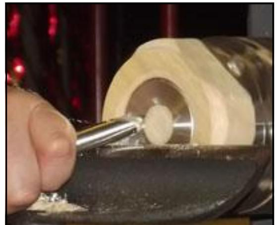
A recess was then cut down the inside of the rim to carry the lid, and the outer end was carefully blended into the first bead on the exterior surface. Having set the depth of the lid recess he completed the interior of the box and sanded / waxed to a final finish.
