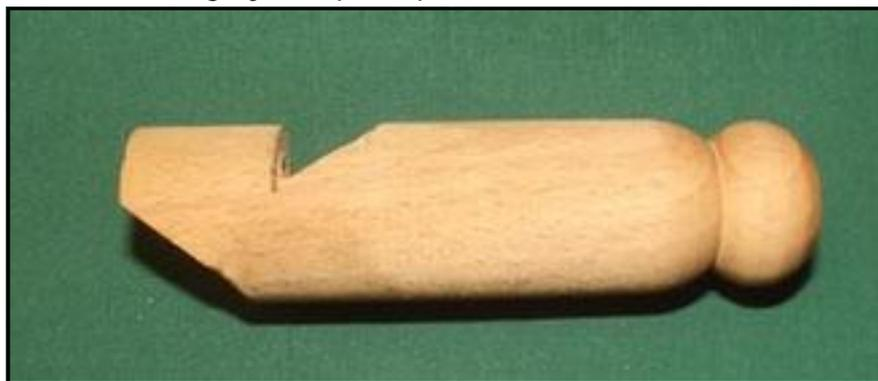
was trued up, and a dimple was put in the centre. A 16mm forstner bit was then used to drill to a depth of 50mm, followed by Simon used a gouge to reduce the wall thickness to about 5mm. Measure 19mm and 31mm from the free end, and saw a notch into the tube,
