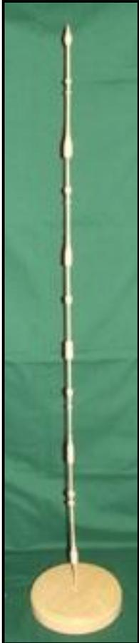
Finally, from Jon Simpson, loosely described as a set of bottles and glasses, the main stem diameter of this trembleur is 2.5mm. The piece started off as an Ash dowel, one metre long and 1/2" diameter, While being turned, it was at one stage, supported by 7 steadies spread along its length. A copy of this will be attempted during the hands on night on July 4th.
