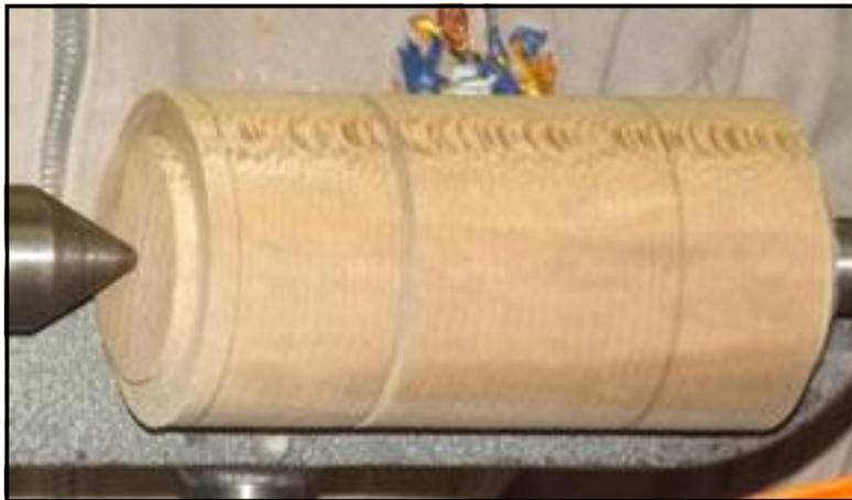
Early in the demonstration Rodger explained that he doesn't know what lathe speed he turns at, you should turn at the fastest speed you can whilst feeling safe. He also explained that for much of this work he uses a skewchi-gouge. More will be said about the tool at the end of this article.
