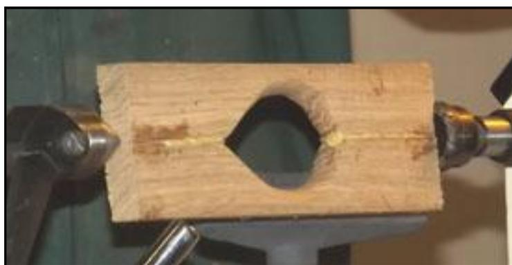
spindle gouge, taking care of the fact that a) there were some hard sharp corners on the move quite close to the tool rest, and b) those corners **MUST** be preserved for gluing up later.
