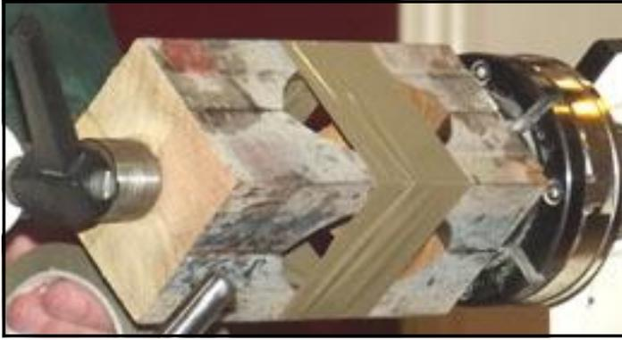
centre. When all is dry, drill the end of the blank to take a metal candle holder. Mount between centres again and wrap packing tape round the centre section to help give a bit of extra support. Cut away the waste at the tail stock end (the top) to form the collar and the candle recess. Next, work on the area near the step centre, cutting away the waste and form a foot for the piece to
