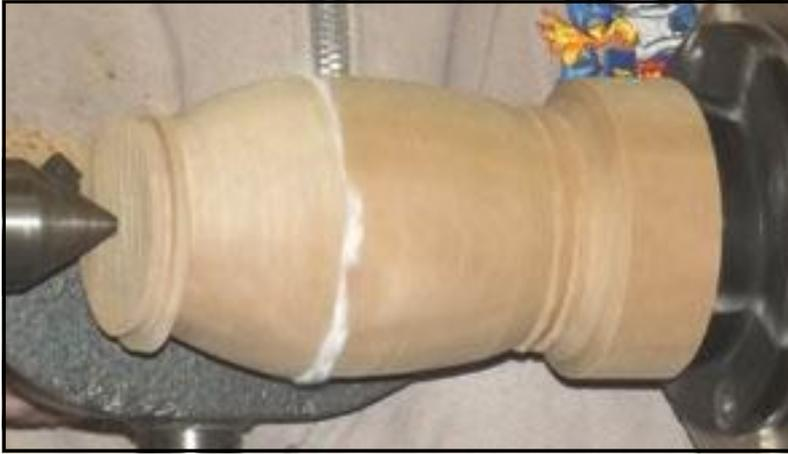
through a similar process, tidy up the end, hollow well into the base and work on the joint recess, ensuring a good fit with the first half. Take very small cuts until you get a good fit.
