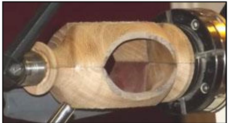
As before, use a 40 grit chisel to get rid of sharp edges. The final stage is to make a jam chuck and reverse the piece, then part off at the base. This is then followed by lots of hand sanding and finishing.
