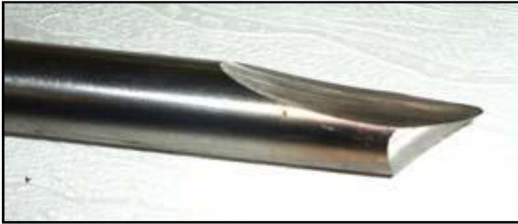
As noted above, Rodger makes a lot of use of a skewchi-gouge. A skewchi-gouge is made from high speed steel bar and is described as a spindle gouge without a flute. When sharpening or re-grinding a skewchi, make sure the top face is concave and has a curved rather than a pointed end. The lower surface
