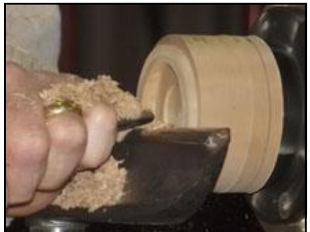
fully. This was followed by the hollowing of the section. For this, use whatever hollowing tool gives you the best results. As you work your way into the piece, you should mirror the internal curve onto the outside.
