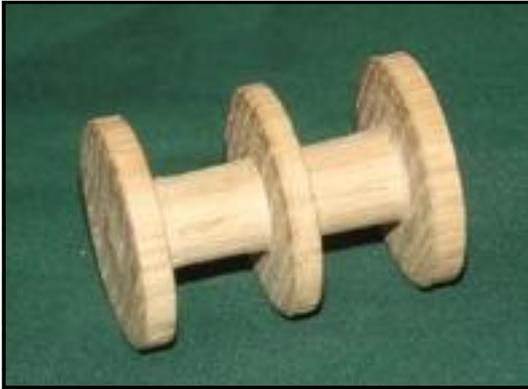
The third piece I demonstrated was a double cotton reel. With a blank mounted in the chuck, round off to about 1" (or less) diameter and make a clean cut across the free end. Starting from the free end, make 5 marks at 1/8", 1/2", 1/8", 1/2", 1/8". Leave the 1/8" sections full diameter, but part in the 2 1/2" sections down to about 1/4" diameter. A quick clean up with 240 and 320 grit, part off, and clean off any remaining pip. Job done. When a customer asks "what's that" you say
