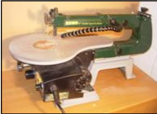
This has been modified to take a saw blade holder conversion kit (much better clamping than the originals).
