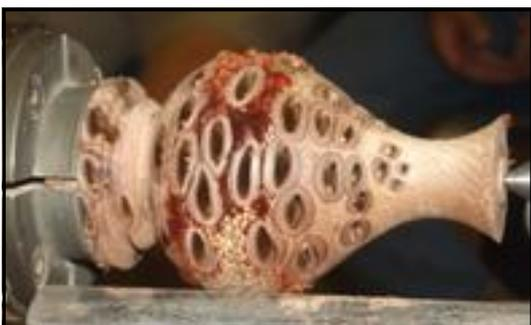
Drill into the end of the piece with a drill bit of suitable diameter, then flair out the neck, sand, seal, polish, part off, done. When you insert the tube, put a small quantity of "Plumbers Mate" on the end to stop it falling out when a potential customers pick it up and turn it over. On pieces like this it is quite practical to fill some of the voids with polyester resin and metal powder to add decoration.
