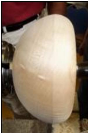
Using both cranked and articulated tools on the left and right side a deep recess was formed under the rim of the piece which was then blended into the exterior of the rim.
