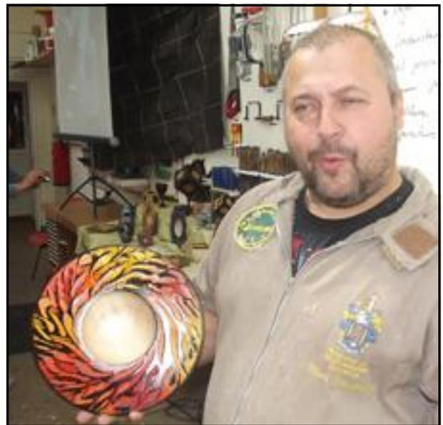
With the piece now mounted in the chuck using the spigot, the centre of the platter was hollowed out, followed by a quick wax and sand. Mick says, "big tools for removing waste wood, small tools for finish cuts".
