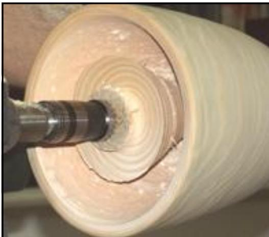
Finish the inside with a scraper. If the timber has moved, slow the lathe down to allow the tool to better follow the surface undulations. Part in at the base with an undercut, shape the base and foot area, and part off. If you are skilled (or brave) add detail to the bottom of the foot before you complete the parting off, otherwise do a bit of reverse chucking and complete the bottom.
