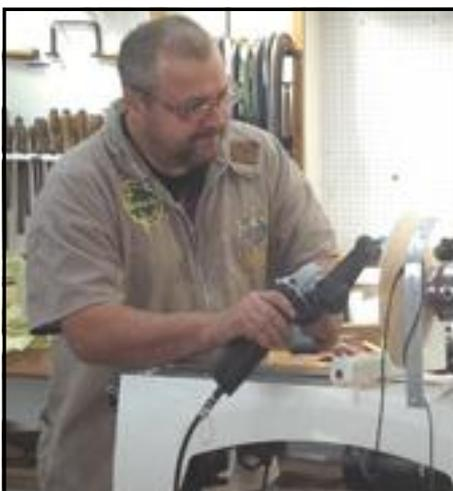
An Arbortec was used to carve deep into the rim section, followed by spray painting with red and yellow stains applied with a diffuser and black acrylic applied with a sponge brush.
