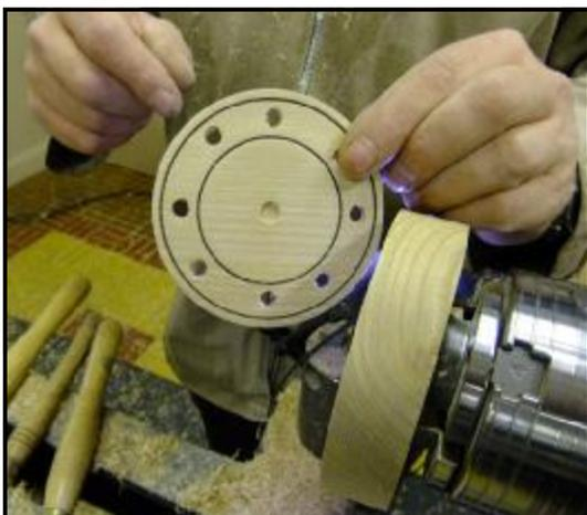
doesn't dig in. He then measured the removed circle with the holes in it in order to make a recess for it to sit in. He stressed how important it was to clean out the swarf before checking the fit. He also explained that a good fit could be ensured by chamfering the cut. If the fit was too loose then some of the front surface could be shaved off. Clean it up and abrade, and perhaps decorate? (Andy is a great fan of pyrography!).
