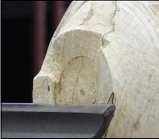
piece of wood to demonstrate with. On the third attempt at getting the large Spalted Beech blank to stay on the lathe, we watched Barry remove the centre section, producing a large section on the lathe, and a smaller section which had been removed from the centre suitable for producing a small low bowl.
