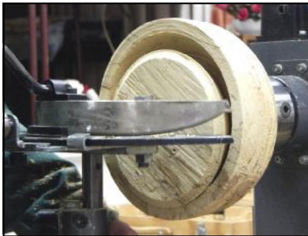
Problem 2: When you are going to use a large blank, make sure your lathe is running in low gear, otherwise it will not have enough torque to overcome the tool pressure you are inventively going to apply.
